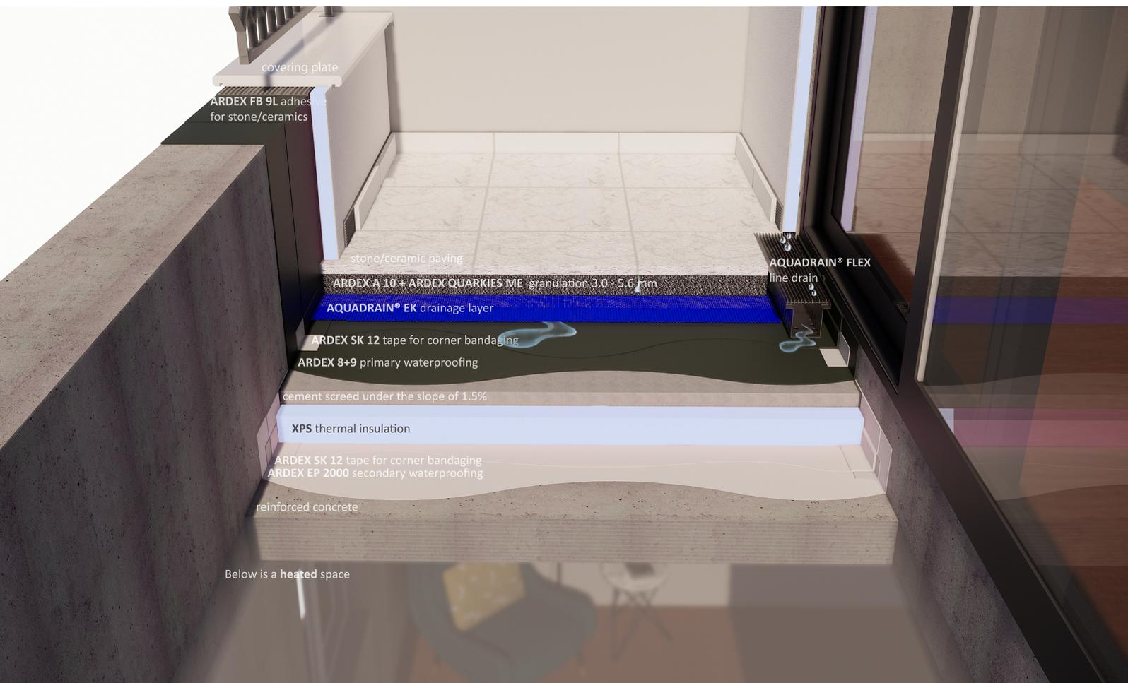
🌱 AquaDrain® EK is drainage system specially made for putting outdoor paving on drainage mortar (ARDEX A10 + ARDEX QUARKIES ME granulation 3.0 – 5.6 mm).
